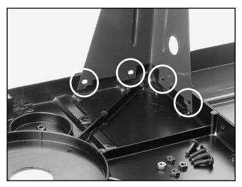
Figure 4. Aligning a leg with the main table.
